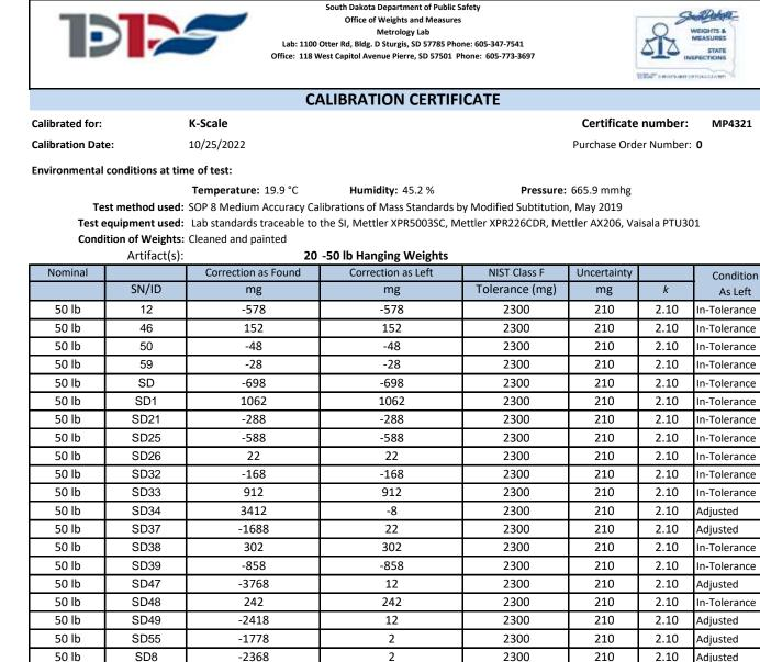
The values reported relate only to those observations made at the time and conditions of the test. This calibration certificate, so numbered, may not be reproduced, except in full, without approval of the laboratory. These weights were not screened for magnetism or checked for density, and effects of magnetism or density are not included in the uncertainties.
